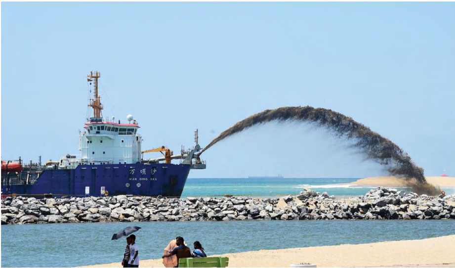
Figure 6. The Wan Qing Sha dredging in the vicinity of Colombo, Sri Lanka. 23
